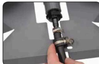
6. Fit padded hose clamp over tubing. (Use 17.5mm clamp for  $\frac{3}{8}$ " tubing or 25.5mm clamp for  $\frac{1}{2}$ " and  $\frac{5}{8}$ " tubing)
