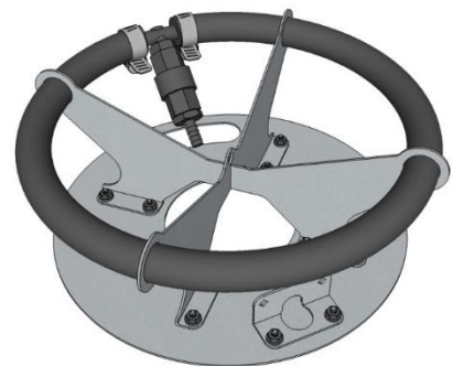
Completed Diffuser Assembly
